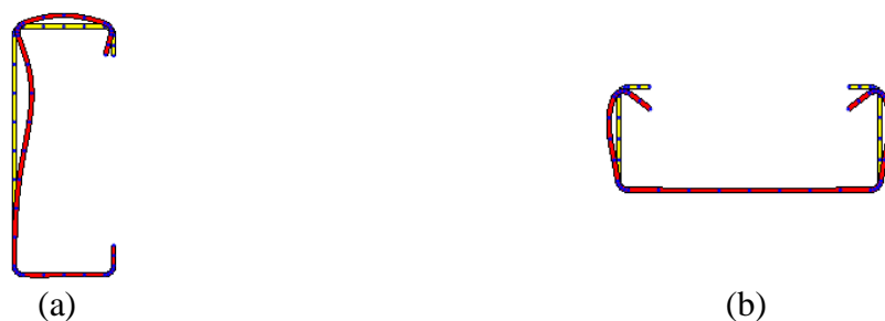
Figure 1. Cross section under local buckling: (a) bending about the major axis; (b) bending about the minor axis.
