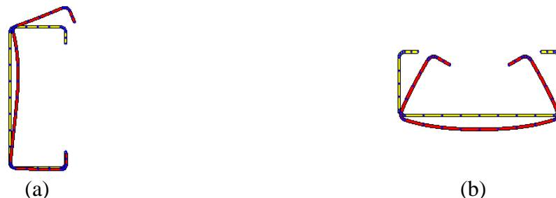
Figure 2. Cross section under distortional buckling: (a) bending about the major axis; (b) bending about the minor axis.
